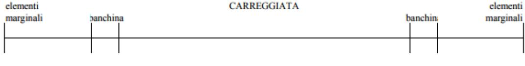
The diagram illustrates a road cross-section. It features a central horizontal line labeled "CARREGGIATA" (carriageway). On either side of the carriageway are two vertical lines labeled "banchina" (shoulder). The area between the outer vertical lines is labeled "PIATTAFORMA STRADALE" (road platform). At the far left and far right ends of the platform, there are additional vertical lines labeled "elementi marginali" (margin elements).
